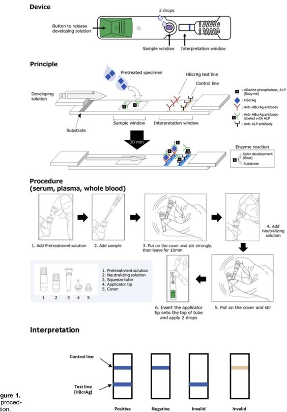
**Supplementary Figure 1.** Device, principle, procedure, and interpretation.
