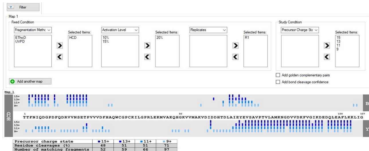
Figure 1: Screenshot of the filter interface of TDFragMapper (top panel) and the visualization module with the corresponding fragmentation map of human Thioredoxin (11 kDa) obtained when varying the precursor charge state in HCD with NCE 20% (bottom panel). Fragmentation maps obtained for larger proteins (21 and 29 kDa) are depicted in Figures S6 and S7.
