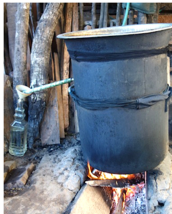
Figure 2. Traditional alcohol production device still in use in the Sayaboury province of Laos.
