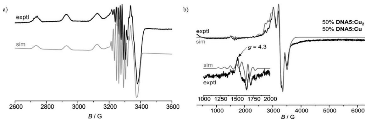
**Figure 27.** (a) X-band CW EPR spectrum of a duplex containing one **Hq-Cu<sup>II</sup>-Hq** metal-base pair overlaid with the simulation (gray). (b) X-band CW EPR spectrum of a duplex containing two consecutive **Hq-Cu<sup>II</sup>-Hq** metal base pairs overlaid with the simulation (gray). Figure taken with permission from Wiley Online Library from reference <sup>18</sup>.
