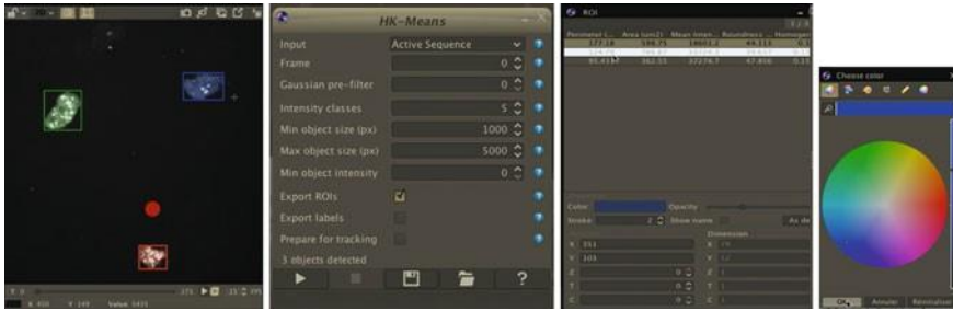
Fig. 25.1 Cell segmentation with HK-Means and ROI color selection. HK-Means can be opened from the detection tab or from the search bar. The first step is to choose which frames we are interested in segmenting (here we select frame 0, but ‘ALL’ is also a possibility). We have to specify the number of intensity classes (see the text for an explanation on HK-Means) in which the histogram is to be split. That is the number of different intercellular intensities (e.g. if all cells are the same intensity, two classes are enough). When in doubt, we recommend choosing higher values, but we also remark that it comes at a computational price. To aid the segmentation of the image into the different classes the user can also input an expected minimum and maximum size for the cells so as to eliminate possible groups that are respectively too small (e.g. debris) or too big to possibly be a cell (e.g. cell clusters). Notice that these sizes are required in pixels, to have a rough idea of the cell size in pixels draw a ROI around the cell and check its size (“Interior” descriptor in the ROI tab at the right-hand side). Finally, applying the Gaussian pre-filter can help improve the segmentation of noisy images. Since the segmentation output are ROIs, we can obtain any descriptor directly from the ROI tab. Here we show the perimeter, the area, the mean intensity, the roundness and the homogeneity inside the ROIs, but many more shape descriptors can be selected using the “gear” button. ROI colors can be chosen (see Tutorial 2)
