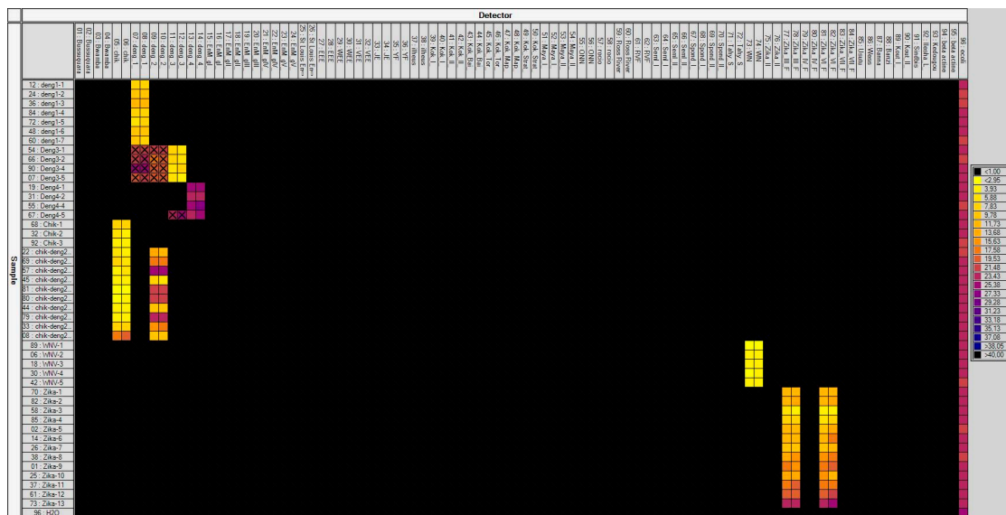
Figure 2. Screening of artificially infected mosquitoes through the BioMark™ dynamic array system developed (96.96 chip). Each square corresponds to a single real-time PCR reaction, where rows indicate the batches of mosquitoes tested and columns represent the targets of each primer/probe set. Crosses indicate cross-reaction of assays. C_t values for each reaction are indicated in color; the corresponding color scale is presented in the legend on the right. The darkest shade of blue and black squares are considered as negative reactions with C_t > 30 . chik: Chikungunya; deng: Dengue; EnM: Murray Encephalitis; St Louis Enc: Saint Louis Encephalitis; EEE: Eastern Equine Encephalitis virus; WEE: Western Equine Encephalitis; VEE: Venezuelan Equine Encephalitis; JE: Japanese Encephalitis; YF: Yellow fever; Kok: Kokobera grou; Maya: Mayaro; ONN: O’nyong nyong; RVF: Rift Valley Fever; Seml: Semliki fores; Spond: Spondweni; Tahy: Tahyna; WN: West Nile; Wess: Wesselsbron; Kout: Koutango.
