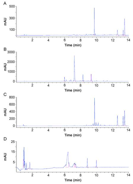
Fig. 1. (A) A typical chromatogram of gentamicin standard solution (USP) (216  $\mu$ g/mL) after OPA derivatization. (B) A typical chromatogram of sisomicin after OPA derivatization (4.65 mg/mL). (C) A typical chromatogram of ALS after OPA derivatization (gentamicin 217  $\mu$ g/mL). (D) Analysis of ALS (gentamicin 217  $\mu$ g/mL) under oxidative conditions (3% H<sub>2</sub>O<sub>2</sub>, 80 °C for 3 h) after OPA derivatization.
