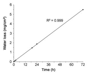
**Fig. 4.** Linear relationship between water loss through TIVAP and time of storage at 40 °C  $\,\pm\,$  2 °C, RH 75%  $\,\pm\,$  5%.
