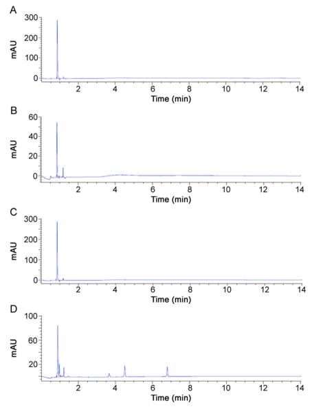
Fig. 2. (A) A typical chromatogram of EDTA-Na<sub>2</sub> (USP) (1.3 mg/mL) after  $CuSO_4$  complexation. (B) A typical chromatogram of nitrilotriacetic acid (43  $\mu$ g/mL) after  $CuSO_4$  complexation. (C) A typical chromatogram of ALS (EDTA-Na<sub>2</sub>: 1.3 mg/mL) under stress oxidative conditions (3%  $H_2O_2$ , 80 °C for 3 h) after  $CuSO_4$  complexation.
