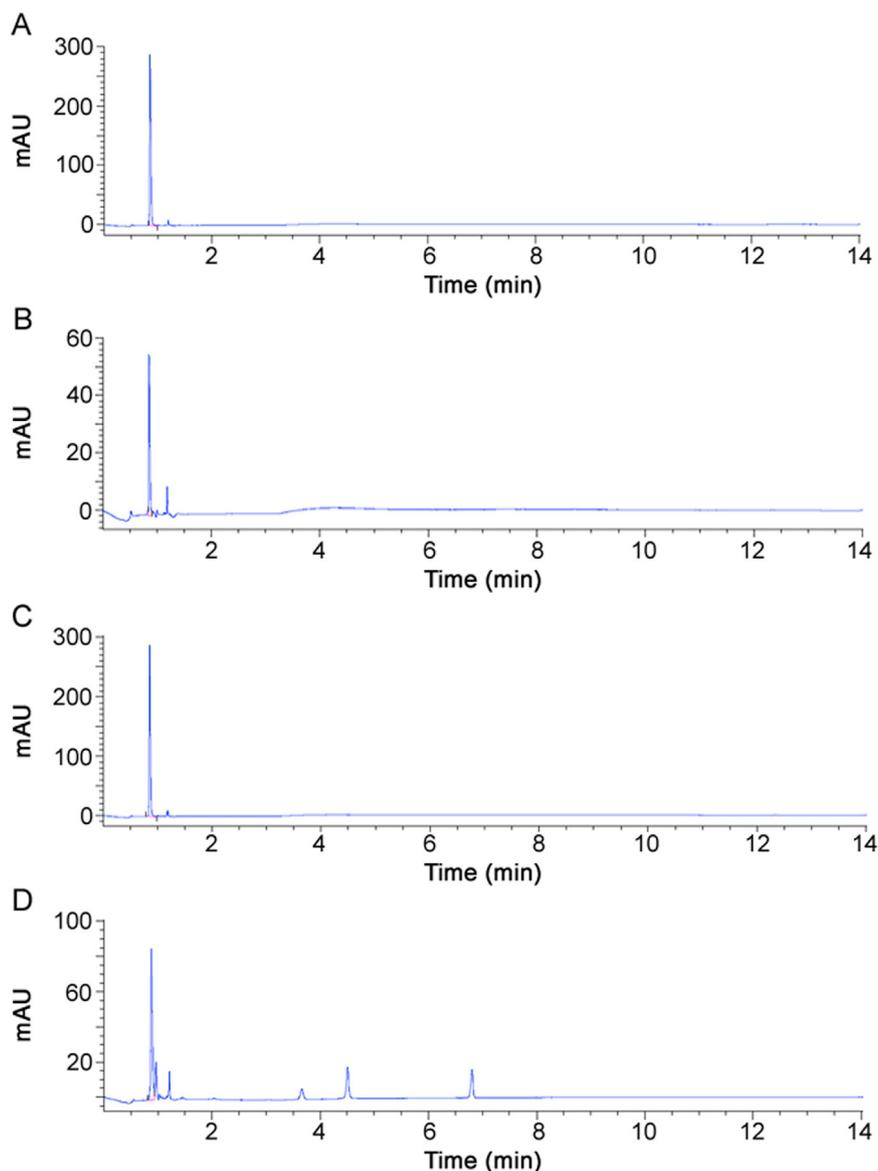
**Fig. 2.** (A) A typical chromatogram of EDTA-Na<sub>2</sub> (USP) (1.3 mg/mL) after CuSO<sub>4</sub> complexation. (B) A typical chromatogram of nitrilotriacetic acid (43 µg/mL) after CuSO<sub>4</sub> complexation. (C) A typical chromatogram of ALS (EDTA-Na<sub>2</sub>: 1.3 mg/mL) after CuSO<sub>4</sub> complexation. (D) Analysis of ALS (EDTA-Na<sub>2</sub>: 1.3 mg/mL) under stress oxidative conditions (3% H<sub>2</sub>O<sub>2</sub>, 80 °C for 3 h) after CuSO<sub>4</sub> complexation.
