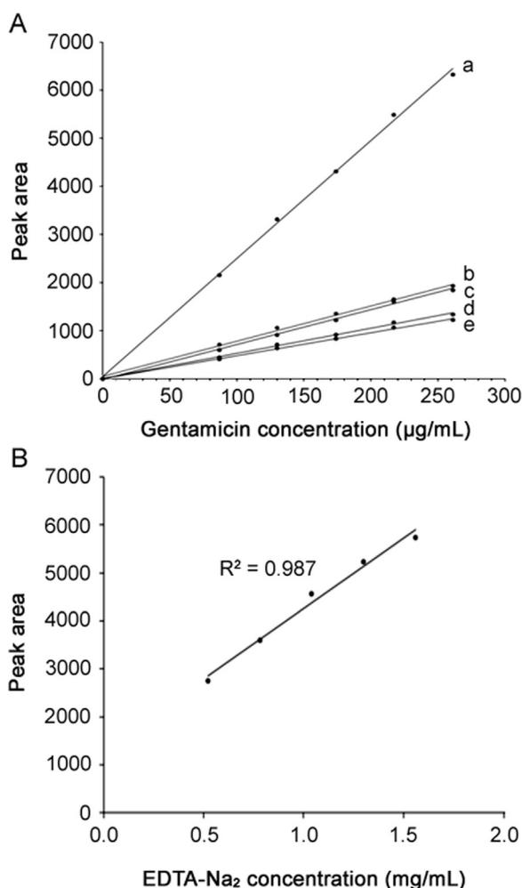
**Fig. 3.** (A) A typical calibration curve of the cumulative peak area (C1, C1a, C2a, C2) of gentamicin sulfate (Panpharma<sup>®</sup>) (a) and four components (b, c, d and e) ranged from 87 to 260 µg/mL (B) A typical EDTA-Na<sub>2</sub> calibration curve ranged from 0.52 to 1.56 mg/mL.
