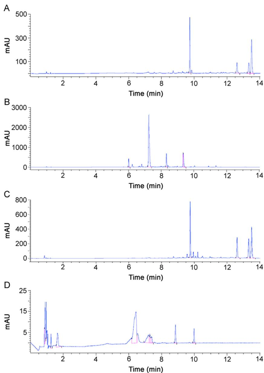
**Fig. 1.** (A) A typical chromatogram of gentamicin standard solution (USP) (216  $\mu$ g/mL) after OPA derivatization. (B) A typical chromatogram of sisomicin after OPA derivatization (4.65 mg/mL). (C) A typical chromatogram of ALS after OPA derivatization (gentamicin 217  $\mu$ g/mL). (D) Analysis of ALS (gentamicin 217  $\mu$ g/mL) under oxidative conditions (3% H<sub>2</sub>O<sub>2</sub>, 80 °C for 3 h) after OPA derivatization.
