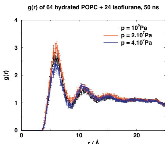
**Figure 5.** Diagram showing the radial distribution function of the C2 atom of isoflurane in the molecular dynamics simulation runs performed with an NPT ensemble. The concentration of isoflurane used is ten times that of clinical concentration.
