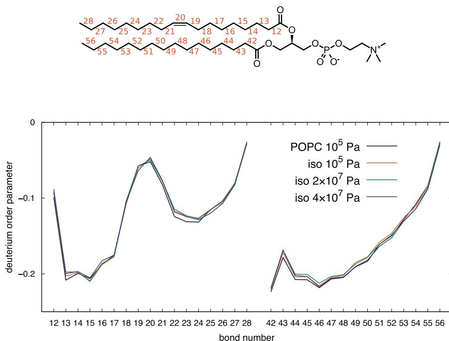
**Figure 7.** The top panel shows the bond numbering scheme used in our calculations. The lower panel shows the bond order parameter of the system consisting of hydrated POPC only (POPC  $10^5$  Pa), and of POPC with isoflurane at three different pressures (iso  $10^5$  Pa, iso  $2 \times 10^7$  Pa and iso  $4 \times 10^7$  Pa).
