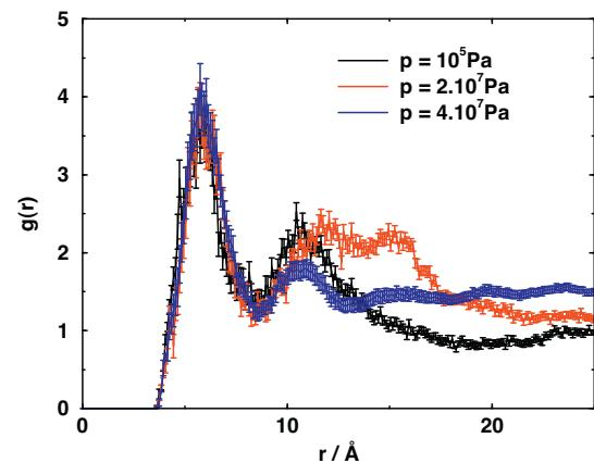
**Figure 3.** Diagram showing the radial distribution function of the C2 atom of isoflurane in the molecular dynamics simulation runs performed with an NPT ensemble. The concentration of isoflurane used is that of clinical concentration.
