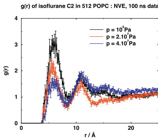
**Figure 4.** Diagram showing the radial distribution function of the C2 atom of isoflurane in the molecular dynamics simulation runs performed with an NVE ensemble. The concentration of isoflurane used is that of clinical concentration.
