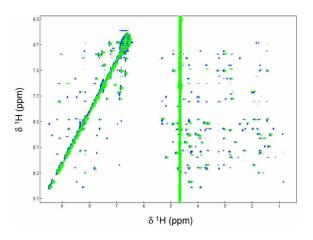
**Figure 2.** Superposition of a region of the NOESY spectra of Pi4 extracted from scorpion venom (green) and obtained by chemical synthesis (blue). Spectra were acquired at 303 K by using a mixing time of 200 msec.
